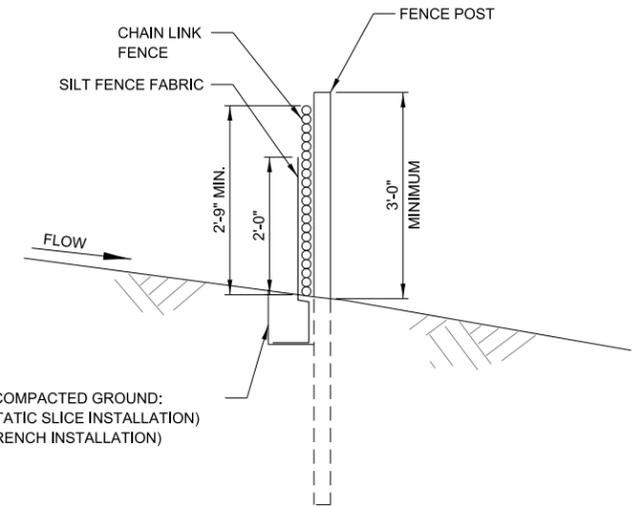
EMBED VERTICALLY INTO COMPACTED GROUND:
